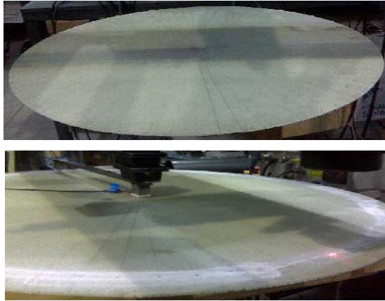
Figure 5: Circular GFRP sample with 5 degree division (top) and with MFCs applied (bottom)
